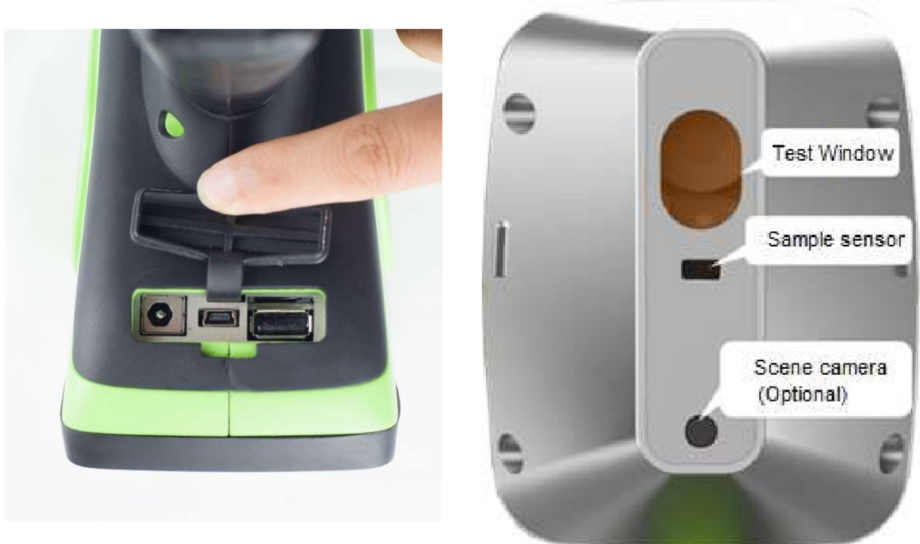
Figure 2. Data interface and test-head components.
