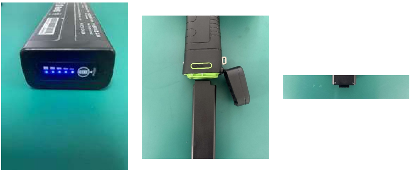
Figure 3. Battery level indication, battery installation and battery lock detail.
