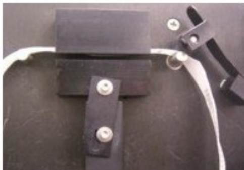
Figure 10A. Actual sensing tape positioned through the detector and pressure-block area.
