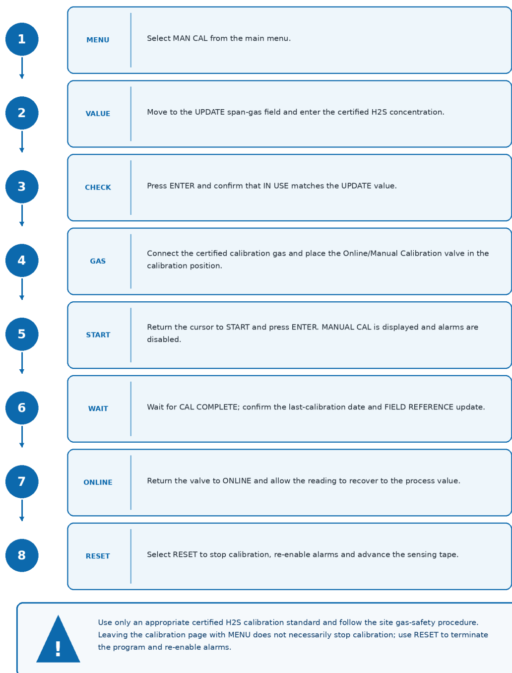
Figure 9 Manual Calibration Workflow
